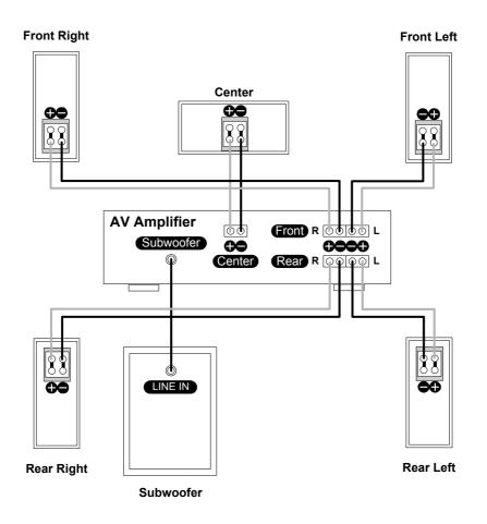
Figure 1. Typical connection of 5.1 channel configuration.
